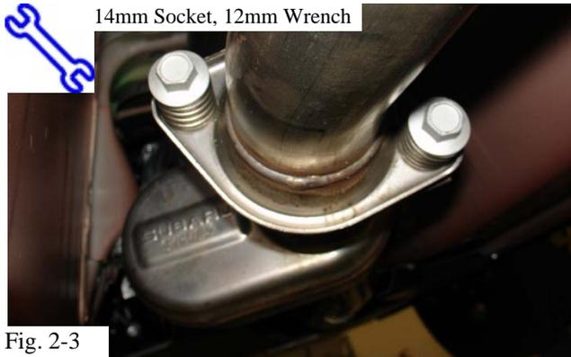
(d) Using a 14mm socket and a 12mm wrench, remove the 2 nuts, bolts and springs from the front flange (Fig. 2-3).
